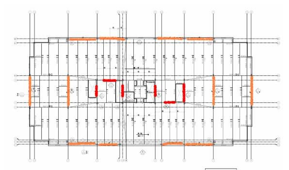
Above is a floor plan with the braces framed highlighted in red and the moment frames highlighted in orange. Below is an elevation of the braced frames.
